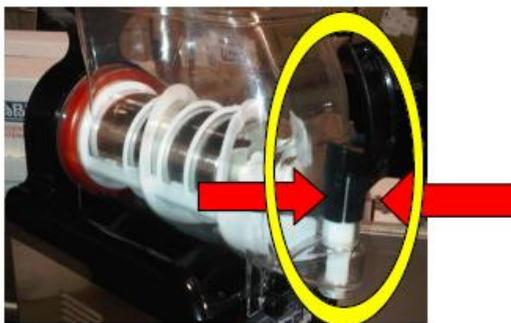
3. Press both sides of the dispensing handle and remove by pulling upwards.
