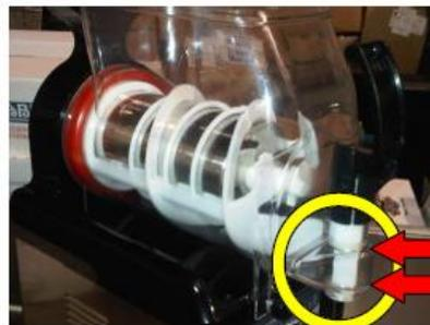
C) Lubricate the around the 2 clean rings on the dispensing handle
