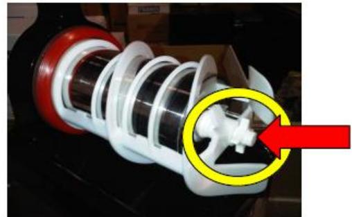
6. Unscrew blade by rotating the front knob clockwise.
