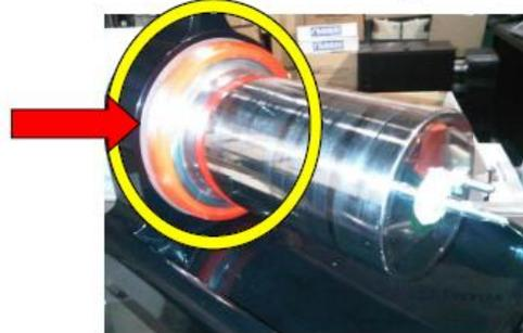
B) Lubricate along the inside and outside of the rear red rubber gasket.
